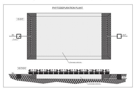
The surface can be fully planted with *Phragmites Australis* or with other marsh varieties. However, it is highly recommendable to select a monoculture option in order to prevent reciprocal infestation. The outlet is always fitted with a well, in a size compatible with incoming and rainwater flow, for housing the timer pump used for redirecting discharge water to the top of the plant when necessary.
